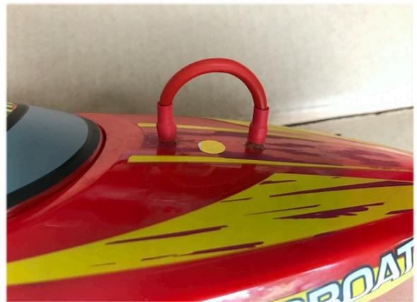
A safety loop or "kill switch" provides the ability to isolate the battery from the ESC & motor from outside the boat. It also acts as a convenient on/off switch without the need to un-tape and remove the hatch cover.
