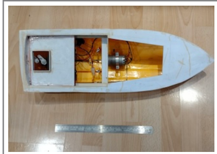
Hull with motor, prop shaft, rudder and propeller
