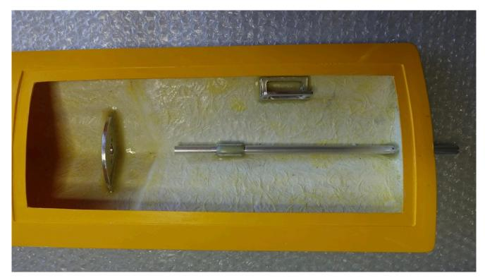
Once the glue was set the transom was drilled for mounting the rudder stand off, turn fin bracket, control rod break through and cooling water break through. The servo mount was then carefully positioned in relation to the break through and rudder arm before gluing in place.
