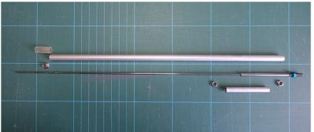
A straight wire drive was selected as the best way forward but commercially available options are limited and expensive so it was decided to custom build a prop shaft around a Tenshock 2mm to 4mm diameter wire & stub shaft drive shaft available from the manufacturer @ \$11.33
