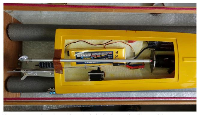
The parts were adjusted to achieve the desired balance point. Once positions were established the prop shaft and tube were marked up in preparation for cutting to length. The positions of the motor mount and servo mount were marked in preparation for fixing later.
