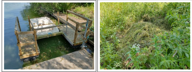
Rescue boat rigged with the weed clearing platform and the first harvest of weed cleared in May
