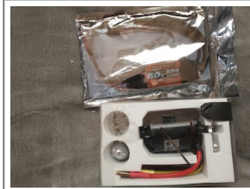
This motor, esc and programming card was bought to power an Aero Kits Patrol Boat.
