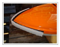
The need for strength, and flexibility, and the construction rules limit the opportunities for weight saving on the hull. But you can use a light waterproof packing material for the bow fender which will not soak up water and add weight like normal sponge rubber would. Motor
