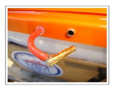
Use wire rated at at least 20 Amps and gold plated connectors from 3.5mm to 4mm diameter. Do not install a fuse as they are resistive. A safety loop made from a short loop of wire and a 4mm gold plated plug & socket connecting the positive of the ESC to the positive of the battery pack will act as a reliable on/off switch. If it is installed outside the hull it allows powering on and powering off without needing access to the inside of the boat.
